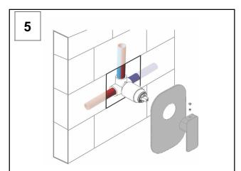
"Decide on a suitable position for the Mixer where all users can operate, determine the route for the incoming cold/hot supply pipe work and the outlet pipe work. Mark an opening sufficient to accommodate the Mixer body, whose dimension is to be smaller than concealing plate (1).
