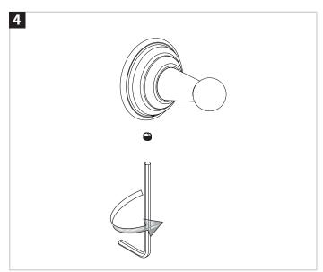
Place accessory over base on the wall and tighten the grub screw in place with a hexagonal key with the grub screw.
