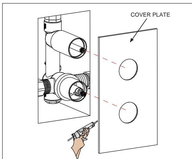
Apply a narrow bead of clear silicone sealant around the back edge of the cover plate and carefully press into position.
