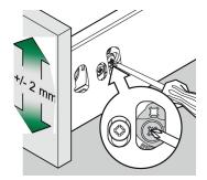
Adjust drawer front by means of eccentric screws.
