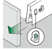
Insert the screwdriver in the left screw and slide it to the left. The drawer front is now released and can be removed.
