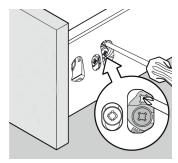
Tighten locking screws.
