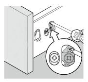
Release locking screws on both sides.
