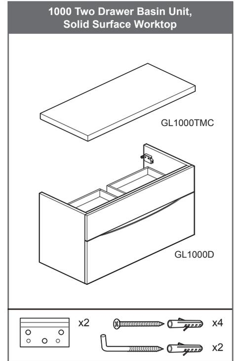
**Tools & equipment needed:** Drill, 8mm Suitable drill bit, Phillips screwdriver, Spirit level, Ruler/tape measure, Pencil, Silicone sealant (clear).
