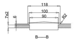
Note: Unless marked, the length, width dimension tolerance should be  $\pm 5$ . The tray thickness dimension tolerance should be ±2.
