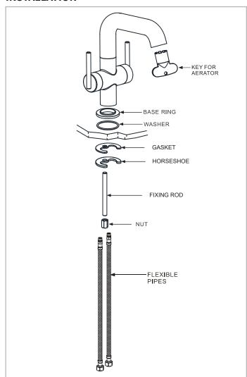
Screw the flexible pipes into the mixer body, and fully hand tighten. Place mixer in position to see if any alteration to the existing supply pipework is necessary. After making any necessary alterations to the pipework, pass the mixer base ring and washer over the flexible pipes and threaded stud to form a seal on sink top. Pass the tails and fixing stud through the hole in the basin from above and place the mixer in position on the basin.
