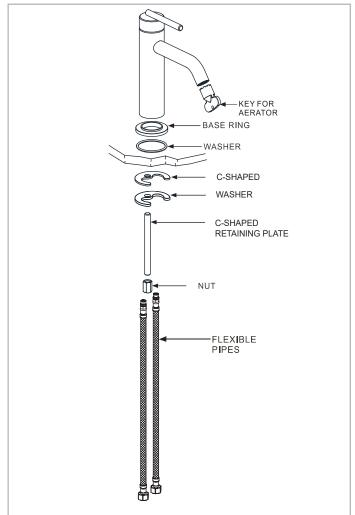
Screw the flexible pipes into the mixer body, and fully hand tighten. Place mixer in position to see if any alteration to the existing supply pipework is necessary. After making any necessary alterations to the pipework, pass the mixer base ring and washer over the flexible pipes and threaded stud to form a seal on sink top. Pass the tails and fixing stud through the hole in the basin from above and place the mixer in position on the basin.
