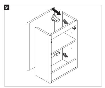
Return the door to the unit by aligning the door hinges to the brackets on the inside of the unit and slide the two components together.
