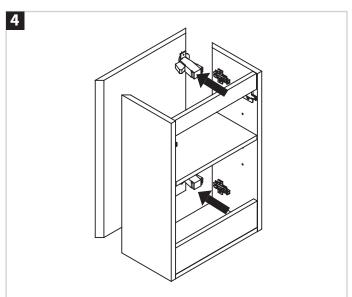
Remove the door from furniture carcass by releasing using the button to the rear of the hinges.
