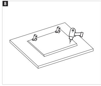
To avoid damaging the door, place the door face down on a composite board. Drill through the pilot hole on the door for the handle you have selected.
