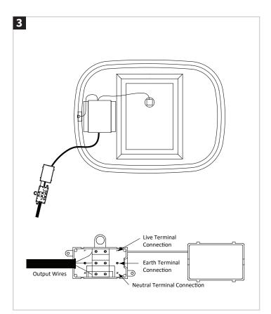
Remove the cover from the electrical connection box. Using a suitable terminal screwdriver make secure connections as follows:
