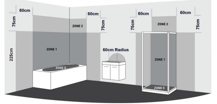
This product is IP44 rated and is suitable for installation within zone 2 above, and complies with the following safety standards:
