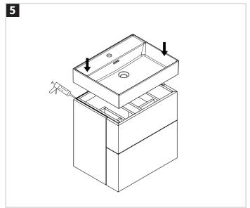
The basin, tap and waste fittings may now be installed, following the manufacturer's instructions. Connect water and waste pipework and turn on the water supply to check for any leaks.
