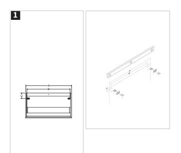
Measure the width and height of the fixing brackets - distances B and C. Mark the wall and prepare to drill.
