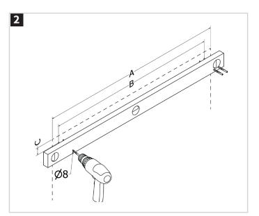
Drill the marks using an 8mm drill bit and ensuring there are no hidden pipes or cables in the wall. Make sure the correct drill bit is used for the surface being drilled and check that the holes are level.
