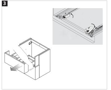
Remove the drawer from the unit by pressing the levers on the underside of each drawer as shown in the diagram. Place the drawer safely aside and ensure it is not dropped or dragged.
