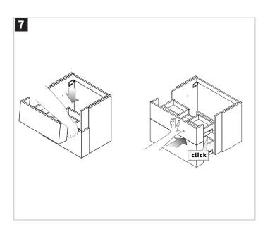
Return the drawers to the unit by extending the drawer guides and placing the drawer on the guides as shown on the diagram. Carefully push the drawer back into the unit until it engages audibly. Check that the drawer is working correctly.
