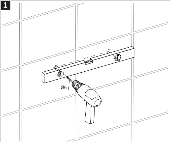
Use a spirit level to ensure the marks are level and drill a pilot hole using a 6mm drill bit suitable for the finished surface (i.e.. Diamond drill bit for ceramic or porcelain tiles)
