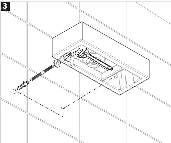
Measure and drill according to the wall fixings being used. Install the basins on the wall with the fixings provided, ensuring the order is as shown in the diagram. The fixings provided are suitable for solid walls only. For any other type of wall please use specialist fixings.
