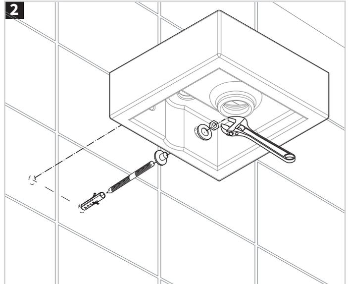
Measure and drill according to the wall fixings being used. Install the basins on the wall with the fixings provided, ensuring the order is as shown in the diagram. The fixings provided are suitable for solid walls only. For any other type of wall please use specialist fixings.
