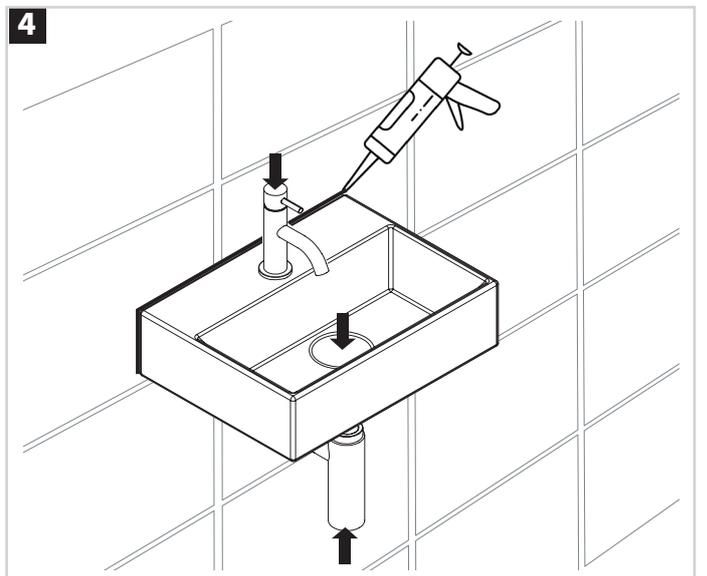
The tap and waste fittings may now be installed, following the manufacturer's instructions. Connect water and waste pipework and turn on the water supply to check for any leaks.
