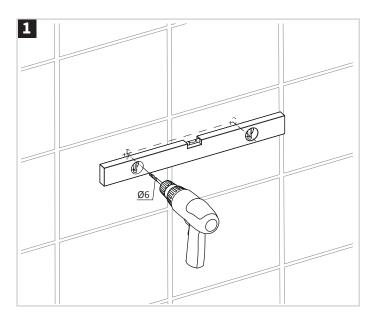
Use a spirit level to ensure the marks are level and drill a pilot hole using a 6mm drill bit suitable for the finished surface (i.e.. Diamond drill bit for ceramic or porcelain tiles)
