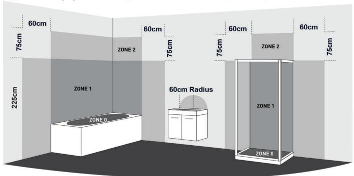
This product is IP44 rated and is suitable for installation within zone 2 above, and complies with the following safety standards:
