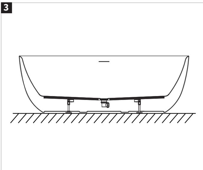
Adjust the legs to ensure they are level with the bottom edge of the bath.
