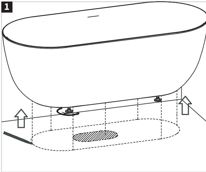
This bath must be installed on a flat and level surface. Remove any humps from the floor before installing. Under floor access is required for plumbing of bath tub waste.
