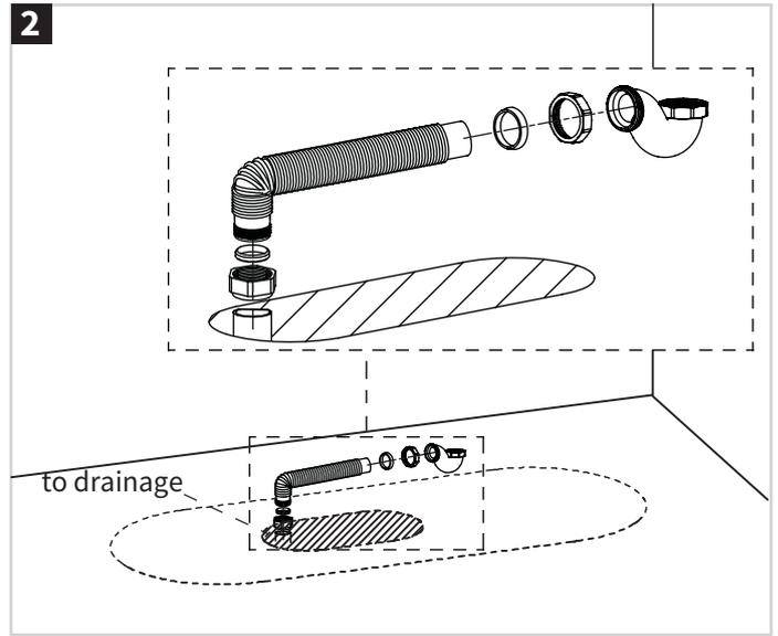
Waste connection is dependant on the site situation; final decision about installation of waste connection should be taken by a suitably qualified person.
