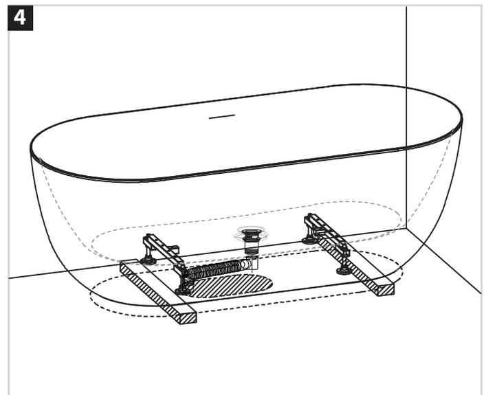
Place the bath on two wooden blocks over the waste connections. Connect the waste. Fill the bath with water and check for leaks from the waste before removing the blocks. Avoid the leg set underneath the bath when you place the bath on two wooden blocks.
