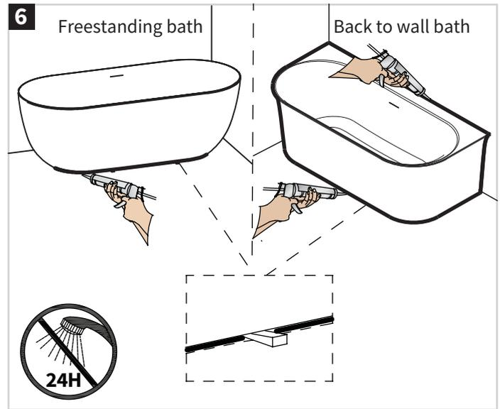
Freestanding bath: Apply a bead of clear silicone sealant around the bottom of the bath to secure it to the floor.
