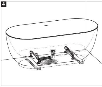
Place the bath on two wooden blocks over the waste connections. Connect the waste. Fill the bath with water and check for leaks from the waste before removing the blocks. Avoid the leg set underneath the bath when you place the bath on two wooden blocks.
