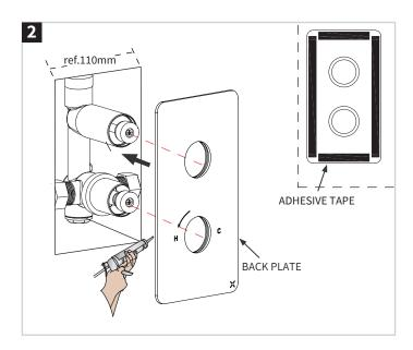
Remove the adhesive tape film on the backside of back plate.
