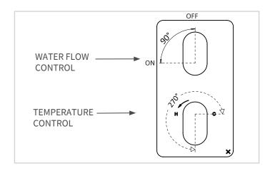
1. Turn the water flow control handle to increase/decrease the water flow and turn on/off.
