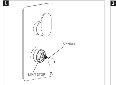
Remove the temperature control handle, metal block. Rotate the exposed thermostatic spindle (clockwise for cold, and anti-clockwise for hot), until the maximum desired showering temperature is set. The suggested maximum pre-set temperature is 42°C.
