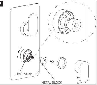
Without any move at the spindle, replace the metal block so that limit stop up to the right hand side of the limit stop on the cartridge. Then refit the temperature control handle.
