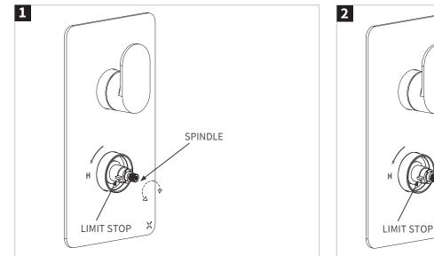
Remove the temperature control handle, metal block. Rotate the exposed thermostatic spindle (clockwise for cold, and anti-clockwise for hot), until the maximum desired showering temperature is set. The suggested maximum pre-set temperature is 42°C.
