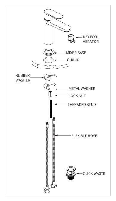
Screw the flexible hoses and threaded stud into the mixer body, and fully hand tighten. Place mixer in position to see if any alteration to the existing supply pipework is necessary. After making any necessary alterations to the pipework, pass the mixer base and o-ring over the flexible hoses and threaded stud to form a seal on sink top. Pass the hoses and fixing stud through the hole in the basin from above and place the mixer in position on the basin.
