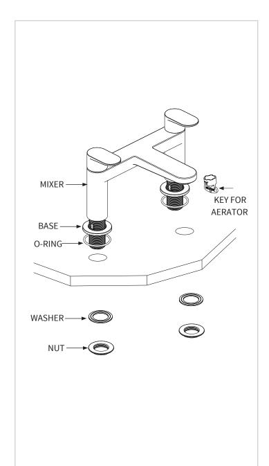
Fit the bases to the mixer body, make sure that the o-rings have been fitted to the bases. Position the assembled body down through the holes of the bath. Fit the washers and nuts onto the threaded part of the body below the bath. Do not over tighten.
