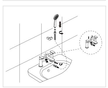
Fit the bases to the mixer body, make sure that the o-rings have been fitted to the bases. Position the assembled body down through the holes of the bath. Fit the washers and nuts onto the threaded part of the body below the bath. Do not over tighten.
