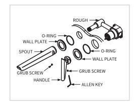
A recess must be made in the wall to accommodate the rough and connections. Place the rough in position (between 40 and 60 mm from the face of the tiles to the back of the rough), check to see if any alterations are needed to the existing pipe work. Secure the set into the recess in the wall.
