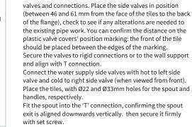
should be placed between the edges of the marking. Secure the valves to rigid connections or to the wall support and align with T connection. Connect the water supply side valves with hot to left side valve and cold to right side valve (when viewed from front). Place the tiles, with Ø22 and Ø33mm holes for the spout and
