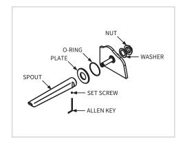
A recess must be made in the wall to accommodate the spout tail. Place the tail in position (between 33 and 73 mm from the face of the tiles to the back of the flange), check to see if any alterations are needed to the existing pipe work. Secure the tail to rigid connections or to other type of connection.
