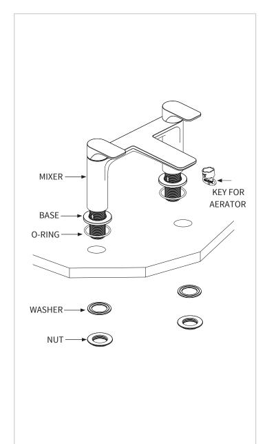
Fit the bases to the mixer body, make sure that the o-rings have been fitted to the bases. Position the assembled body down through the holes of the bath. Fit the washers and nuts onto the threaded part of the body below the bath. Do not over tighten.
