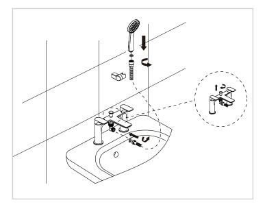
Fit the bases to the mixer body, make sure that the o-rings have been fitted to the bases. Position the assembled body down through the holes of the bath. Fit the washers and nuts onto the threaded part of the body below the bath. Do not over tighten.
