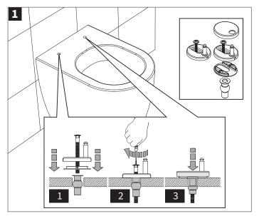
Locate the fixings on the toilet seat and tighten in the order shown, using a screw driver. Do not over-tighten at this stage.
