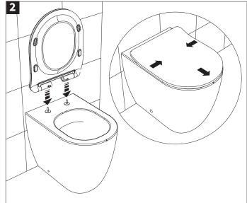
Insert the toilet seat into the fixings and allow to soft-close. Move the seat into position, ensuring the sides and front are flush with the toilet.
