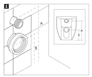
Follow the manufacturer's instructions for the installation of the concealed cistern selected, ensuring the inlet and outlet wastes match the measurements of the back to wall toilet.
