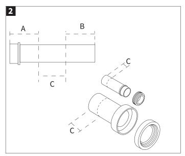
Push the inlet as far as possible into the toilet and mark the distance on the pipe. Measurement A.
