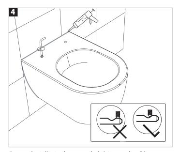
Secure the toilet to the concealed cistern and wall by tightening the grub screws to the bullet fixings.
