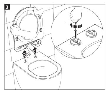
Once the position of the toilet seat is achieved, carefully remove the toilet seat by pressing the central release button. Avoid moving the fixings whilst releasing the seat and tighten the fixings using a screw driver and moderate force. The Cover caps can now be applied before returning the seat to its position.
