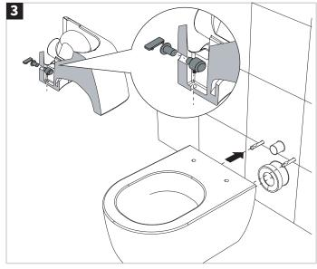
Place the toilet upside down and assemble the fixing kit on the toilet installation holes ensuring a tight fit. The grub screws should be facing up, so they can be accessed through the toilet seat holes.
