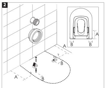
Offer the toilet to its position and mark the location of the side holes on the floor. Then remove the toilet and measure the thickness of the ceramic at distance A. Install the toilet floor fixings.
