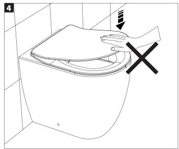
Do not force the toilet seat shut as this may damage the softclose mechanism over time. Do not stand on the seat. When cleaning the toilet, always leave the toilet seat open to allow chemical gases to release. Do not leave harsh chemicals in the toilet bowl with the seat lid closed.
