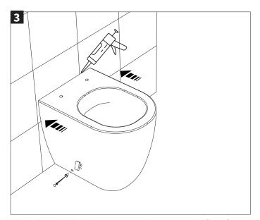
Place the toilet back in position and secure to the floor fixings using the screws, washers and cover caps provided.
