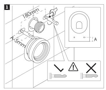
Follow the manufacturer's instructions for the installation of the concealed cistern selected, ensuring the fixing points match the width of the wall hung toilet.
