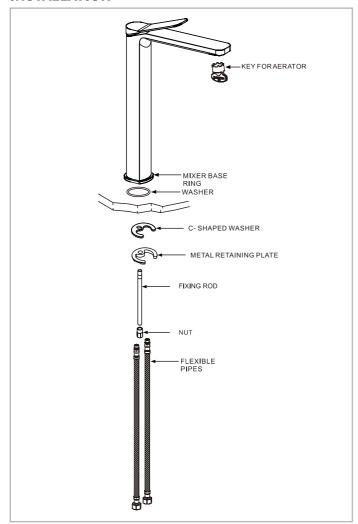
Screw the flexible pipes into the mixer body, and fully hand tighten. Place mixer in position to see if any alteration to the existing supply pipework is necessary. After making any necessary alterations to the pipework, pass the mixer base ring and washer over the flexible pipes and threaded stud to form a seal on basin top. Pass the tails and fixing stud through the hole in the basin from above and place the mixer in position on the basin.
