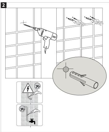
Carefully drill the required holes and insert wall plugs. Note screws and plugs supplied are suitable for solid walls only.
