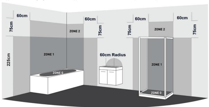
This product is IP44 rated and is suitable for installation within zone 2 above, and complies with the following safety standards:
