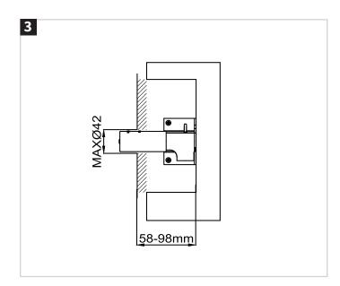
Don't remove plastic cover on the built-in tap, until the wall is completely finished; when tiles have set, remove the plastic cover.
