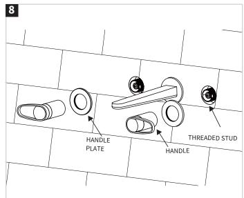
Set the handle plate in position, then screw handle into the threaded stud, and tighten the handle. Please make sure the two handles are aligned and the lateral direction are "OFF".
