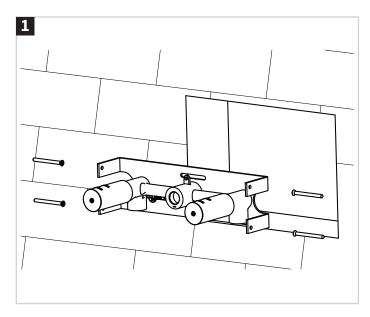
Flush the piping with plenty of water prior to installation. **IMPORTANT!** The trim set needs to be used with UB-130ROUGH.
