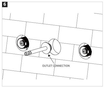
Screw and seal the outlet connection to the body on the wall.
