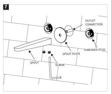
Slide the spout plate over the outlet connection to make it close to the wall, insert the spout onto the valve body and tighten it with the grub screws taking care not to damage the surface of the spout.
