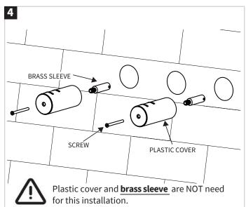
Unscrew the screws of plastic cover with a properly sized screwdrive. Remove the plastic cover and **brass sleeve** from the valve.
