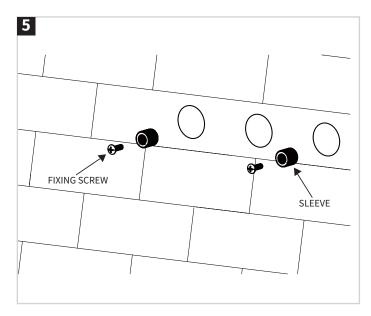
Attach the **sleeve** to the threaded stud using the fixing screws to fix them (in spare bag). These allow the two handles to align better.
