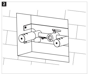
Place the bracket and valve body in position and determine what alteration to the existing pipework is necessary. Secure the bracket using suitable fixing screws for the wall type.
