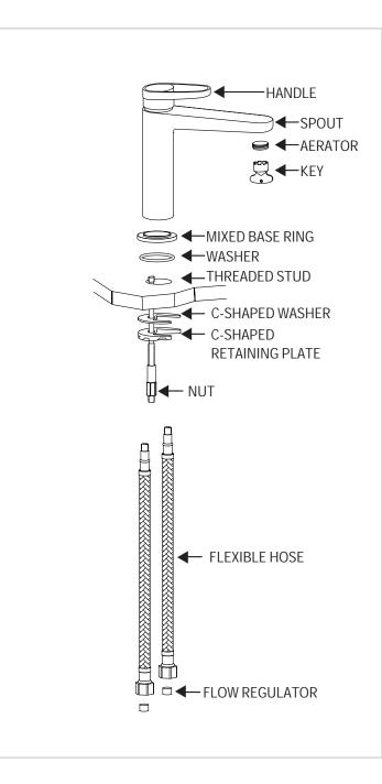
Screw the flexible pipes into the mixer body, and fully hand tighten. Place mixer in position to see if any alteration to the existing supply pipework is necessary. After making any necessary alterations to the pipework, pass the mixer base ring and washer over the flexible pipes and threaded stud to form a seal on sink top. Pass the tails and fixing stud through the hole in the basin from above and place the mixer in position on the basin.
