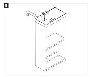
Apply silicone sealant at the back and top of the basin and unit to keep watertight. Check the manufacturer's instructions for drying times. Connect water and waste pipework and turn on the water supply to check for any leaks.
