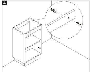
Drill the marks using an 8mm drill bit and ensuring there are no hidden pipes or cables in the wall. Make sure the correct drill bit is used for the surface being drilled and check that the holes are level. Insert appropriate wall plugs, replace the unit and secure using supplied fixing screws.
