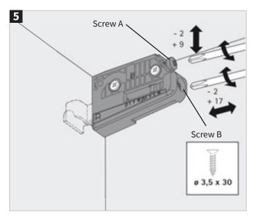
Adjust the level and height of cabinet using adjustment screw A. Once cabinet is level fully tighten screw B.
