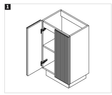
Before installation remove door or doors by pressing the lever at the rear of the hinge. Place doors on a soft surface to protect. The shelf can also be removed to aid installation.
