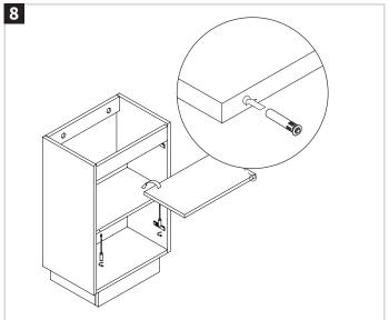
Please note the shelf will also need to be rotated through 180 degrees and the push open mechanism moved to the front and open side of the door.
