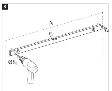
Floorstanding units must be secured to the wall via the rear bracing bar. Once the unit is correctly positioned mark suitable fixing locations on the bracing bar. Drill through the bracing bar and mark corresponding locations on the wall. Remove the unit and place to one side.
