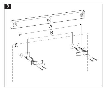
Mark appropriate positions for fixing brackets on a level line. Drill holes using appropriate bit and insert fixings suitable for wall type. Loosen fixing brackets on unit and attach to wall fixings. Adjust for height and level using the adjustment screws. Fully tighten once correctly positioned.
