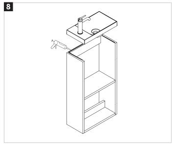
We recommend fitting the tap and waste to the basin before the basin is fitted to the unit. Place basin on unit with a bed of silicone to secure.
