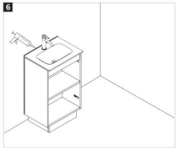
The tap and waste fittings may now be connected, following the manufacturer's instructions. Turn on the water supply to check for any leaks. Important: Apply silicone sealant. Check the manufacturer's instructions for drying times.
