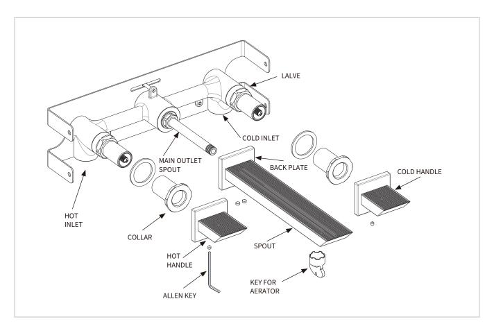
First shut off your water heating system then, with your mains stop cockclosed, open the lowest hot and cold taps in the house and allow to rununtil the cold storage tank and pipes are empty (the hot water storagecylinder always remains full). Fitting isolating valves to the inlet feeds is recommended for ease ofmaintenance.
