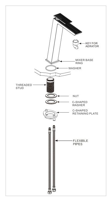
Screw the flexible pipes into the mixer body, and fully hand tighten. Place mixer in position to see if any alteration to the existing supply pipework is necessary. After making any necessary alterations to the pipework, pass the mixer base ring and washer over the flexible pipes and threaded stud to form a seal on sink top. Pass the tails and fixing stud through the hole in the basin from above and place the mixer in position on the basin.
