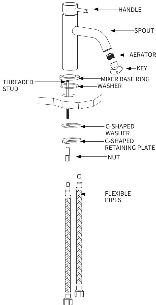
Screw the flexible pipes into the mixer body, and fully hand tighten. Place mixer in position to see if any alteration to the existing supply pipework is necessary. After making any necessary alterations to the pipework, pass the mixer base ring and washer over the flexible pipes and threaded stud to form a seal on sink top. Pass the tails and fixing stud through the hole in the basin from above and place the mixer in position on the basin.
