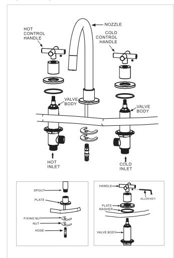
First shut off your water heating system then, with your mains stop cock closed, open the lowest hot and cold taps in the house and allow to run until the cold storage tank and pipes are empty (the hot water storage cylinder always remains full). Where combination boilers are fitted it is only necessary to turn of the boiler and shut off the incoming mains. Fitting isolating valves to the inlet feeds is recommended for ease of maintenance.
