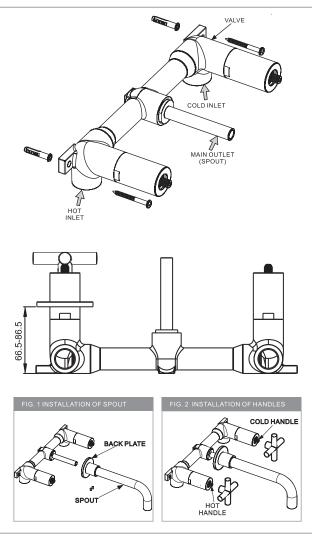
First shut off your water heating system then, with your mains stop cock closed, open the lowest hot and cold taps in the house and allow to run until the cold storage tank and pipes are empty (the hot water storage cylinder always remains full). Where combination boilers are fitted it is only necessary to turn of the boiler and shut off the incoming mains. Fitting isolating valves to the inlet feeds is recommended for ease of maintenance.
