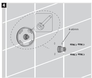
Mark the positions of the screw holes. Remove the mounting plate and drill the holes (4-ø6mm)to install wall plugs.
