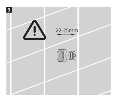
Attention: Ensure the exposed part should be between 22 to 25 mm from the tile to the end of connector.
