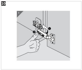
Snap the hinge onto the front of the base and press on the back
