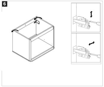
With the wall brackets firmly installed on the wall and level, the unit carcass can now be mounted on the wall brackets and adjusted to ensure it is flush with the wall and level
