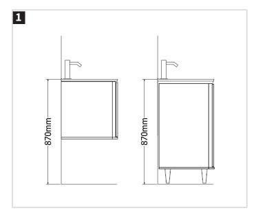
Determine the position and height of the unit, ensuring the recommended heights are followed. Ensure the measurements and markings you make are straight. Check that the plumbing connections from the wall are within the void provided.
