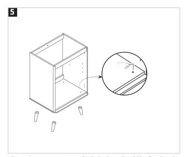
This is the correct way in which the legs should be fixed to the floor of the furniture.
