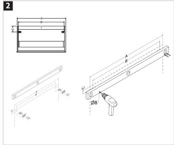
Measure the width and height of the fixing brackets - distances B and C. Mark the wall and prepare to drill.
