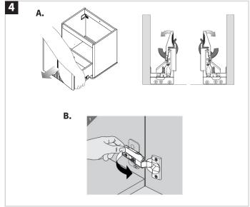
A. Remove the drawer from the unit by pressing the levers on the underside of each drawer as shown in the diagram. Place the drawer safely aside and ensure it is not dropped or dragged.
