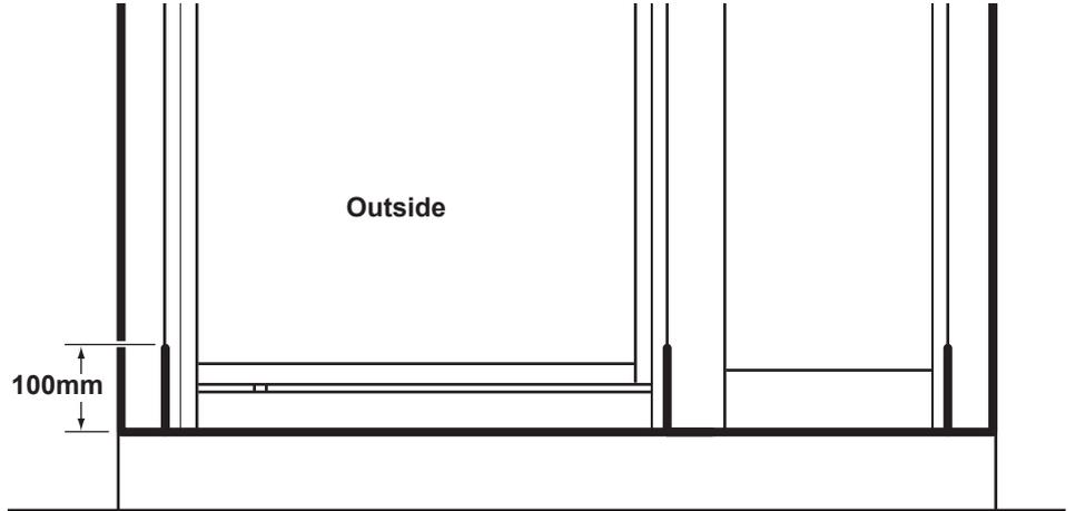
**Sealing outside:** Run a line of silicone sealant from top to bottom down the joint between the wall channels and tiles. Run a line of silicone sealant 100mm up the joint where the door/inline panel slots into the wall channels and where the door slots into the inline panel. Run a line of sealant along the base in the joint between the bottom of the enclosure and the tray, from wall to wall.
