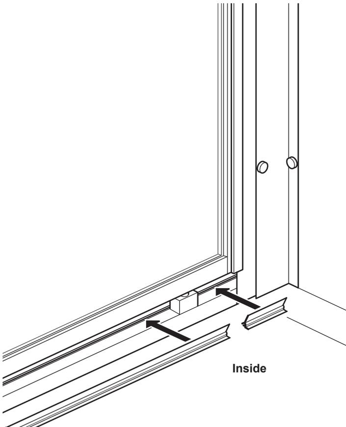
**Optional:** It is only necessary to fit the plastic Anti splash strip (E) if water splashes out through the gap under the door. Cut the strip to size (using scissors) and push fit onto the lug shown on the bottom door frame as shown.
