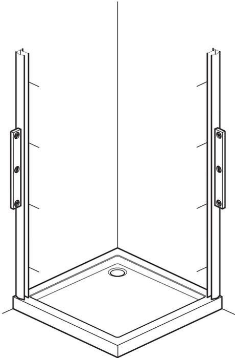
Remove both wall channels from the door frame. Place each wall channel in position on the tray (10 - 15mm in from the outer edges of the tray), use a spirit level to ensure they are vertical and mark all 8 fixing holes onto the walls (holes inside).
