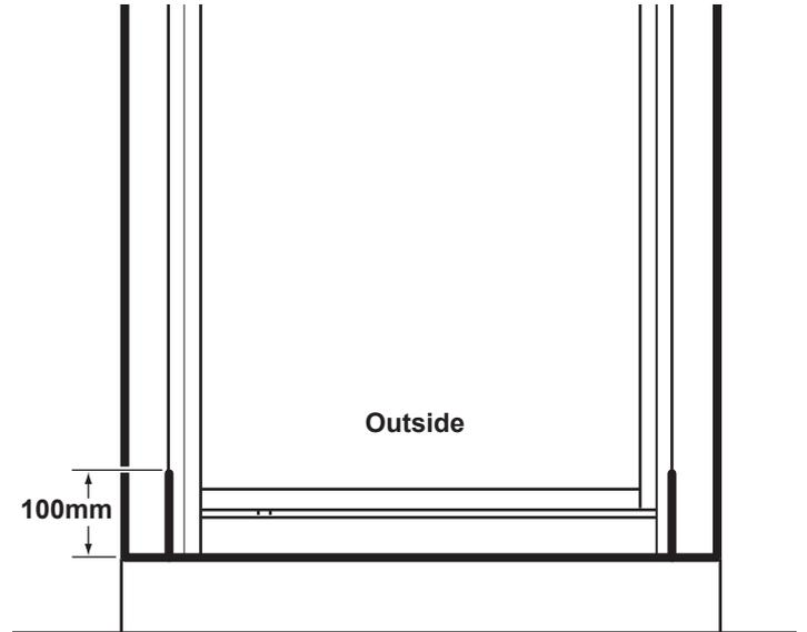
**Sealing outside:** Run a line of silicone sealant from top to bottom down the joint between the wall channels and tiles. Run a line of silicone sealant 100mm up the joint where the door slots into the wall channels. Run a line of sealant along the base in the joint between the bottom of the enclosure and the tray, from wall to wall.
