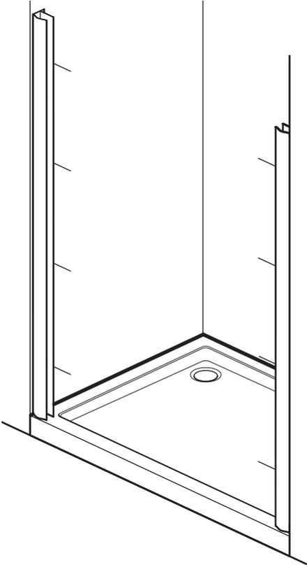
Remove both wall channels from the door frame. Place each wall channel in position on the tray (10 - 15mm in from the outer edge of the tray), ensure they are vertical and mark all 8 fixing holes onto the walls (holes inside).
