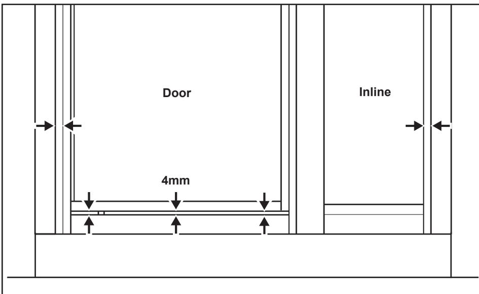
Centre the door/inline panel between the wall channels.
