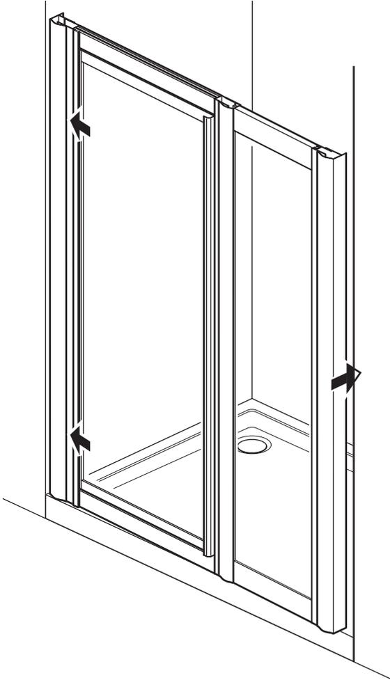
Carefully insert the door/inline panel into the 'fixed' wall channel and swing the free end into position on the opposite wall.
