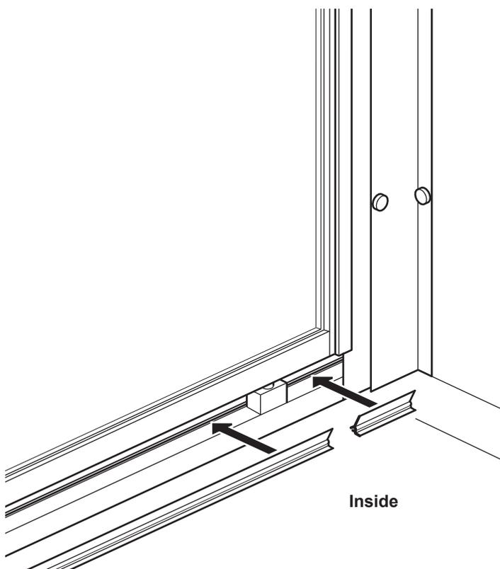
**Optional:** It is only necessary to fit the plastic Anti splash strip (E) if water splashes out through the gap under the door. Cut the strip to size (using scissors) and push fit onto the lug shown on the bottom door frame as shown. **Note:** If the anti splash strip catches on the door, simply trim to fit.
