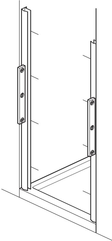
Remove both wall channels from the door frame. Place each wall channel in position on the tray (10 - 15mm in from the outer edge of the tray), use a spirit level to ensure they are vertical and mark all 8 fixing holes onto the walls (holes inside).
