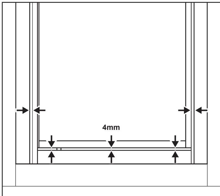
**Before fixing the door to the wall channels you must make sure that the door is square within its outer frame.**
