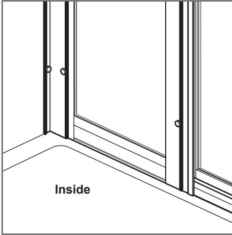
**Sealing inside:** Run a line of silicone sealant from top to bottom down the joint between the wall channels and tiles. Run a line of silicone sealant from top to bottom down the joint where the door/inline panel slots into the wall channels and where the door slots into the inline panel. **Do not seal the enclosure to the tray on the inside.**
