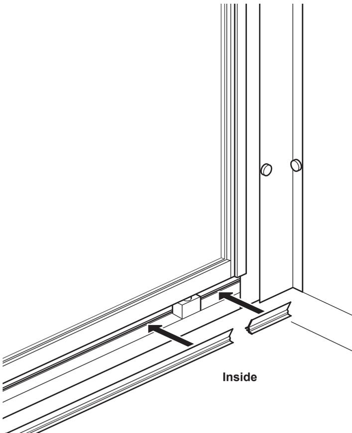
**Optional:** It is only necessary to fit the plastic Anti splash strip (E) if water splashes out through the gap under the door. Cut the strip to size (using scissors) and push fit onto the lug shown on the bottom door frame as shown. **Note:** If the anti splash strip catches on the door, simply trim to fit.
