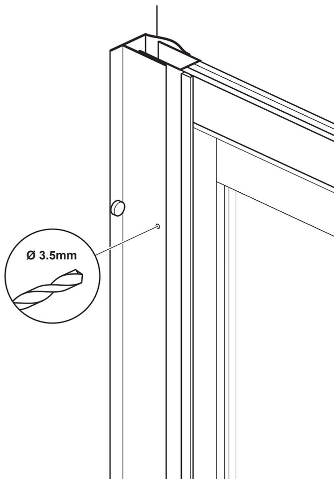
Once you have checked that the door opens and closes correctly fix the door to the wall channels.
