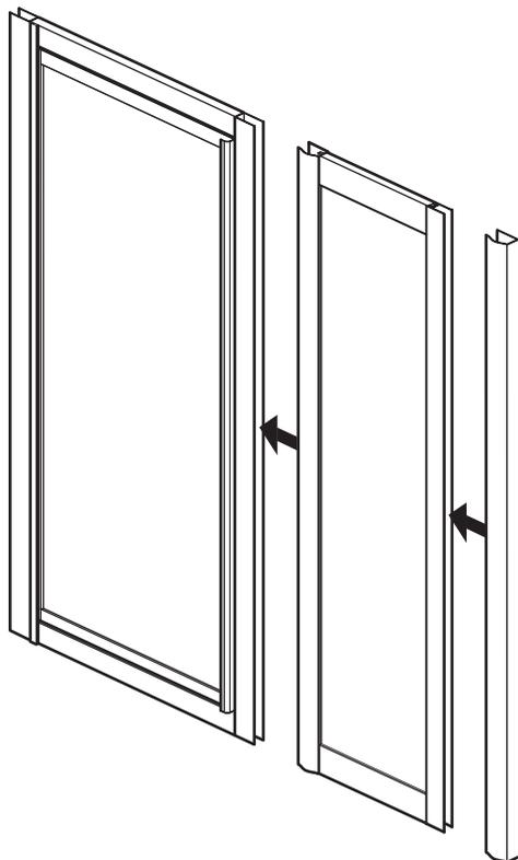
Push the remaining wall channel onto the flat side of the inline panel, then fully push the other side of the inline panel onto the opening/handle side of the door.
