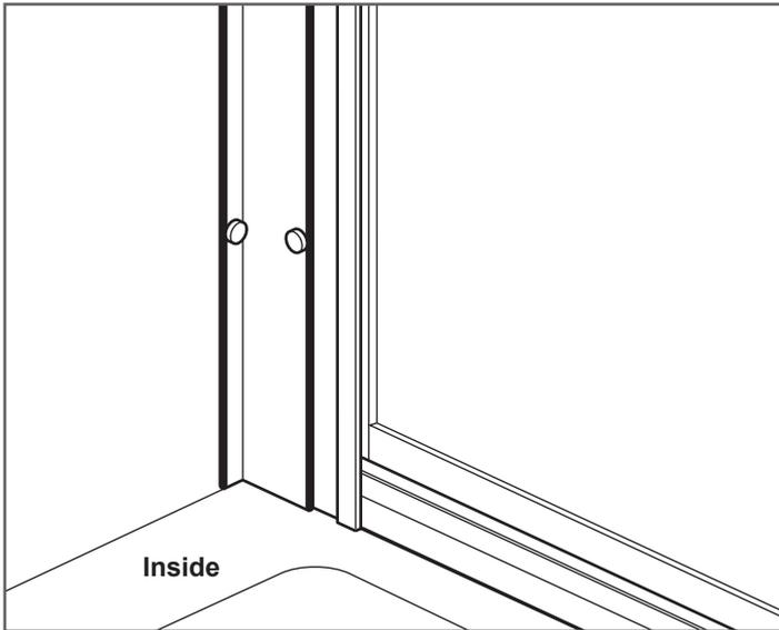
**Sealing inside:** Run a line of silicone sealant from top to bottom down the joint between the wall channels and tiles, also down the joint where the door slots into the wall channels.
