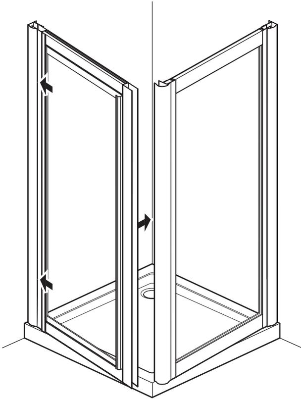
Insert the door into the other wall channel and swing the free end into position on the tray. Push the corner post, fixed to the side panel, onto the side of the door.
