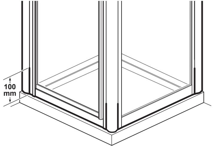
**Sealing inside:** Run a line of silicone sealant from top to bottom down the joint between the wall channels and tiles. Run a line of silicone sealant from top to bottom down the joint where the door and side panel slot into the wall channels and the door slots into the centre post.
