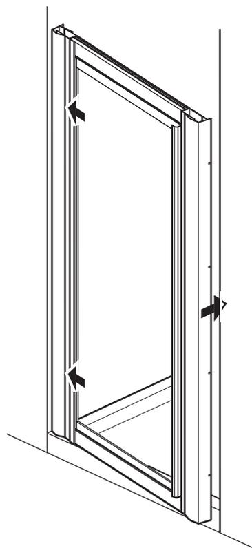
Push the remaining wall channel back onto the door frame on the opening/handle side of the door.
