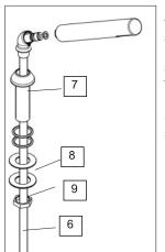
border of bath-tube. Working below the border, insert the special gasket and washer (8), the nut (9), tighten having care to position correctly the shower. Connect the flexible hose at the spout.
