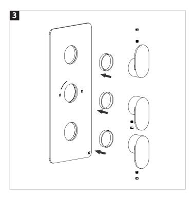
Assemble the handles and the plastic rings. The plastic ring must be placed between the sleeve and the handle.
