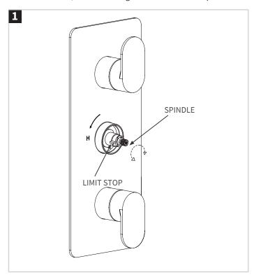
Remove the temperature control handle, metal block. Rotate the exposed thermostatic spindle (clockwise for cold, and anti-clockwise for hot), until the maximum desired showering temperature is set. The suggested maximum pre-set temperature is 42°C.
