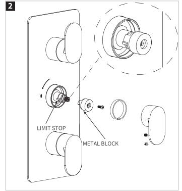
Without any move at the spindle, replace the metal block so that limit stop up to the right hand side of the limit stop on the cartridge. Then refit the temperature control handle.
