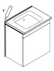
**Note:** Basin waste and taps fittings when over tightened can create stress within the basin material which may in time cause the failure of the product. Waste fittings should be carefully bedded in silicone and the back nut hang tightened an additional quarter turn using a suitable spanner is sufficient to create the required waterlight seal. Care should also be taken when fitting brassware to tap platforms in order to prevent similar stress related failures
