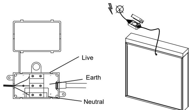
Close the connection box cover. Restore the mains supply and test the function of the lights and shaver socket. See operating instructions below.
