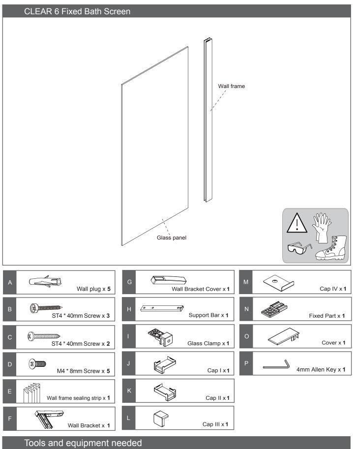
Drill, 6mm Masonry drill bit, 3.2mm General drill bit, Philips screwdriver, Spirit level, Pencil, Scissors, Silicone sealant.
