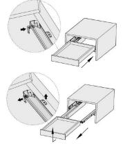
Pull out the drawer to its full extension, gently squeeze the locking levers outwards on both sides and pull the drawer off the runners at the front.
