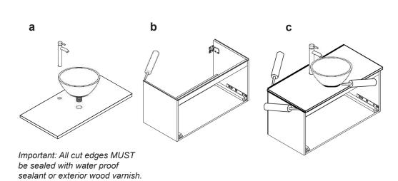
**a:** Prepare worktop for tap/s and basin. Cut holes where required using a suitable sized hole cutter to suit the basin waste diameter, tao fitting and worktop material.
