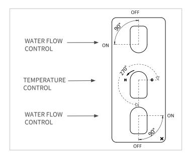
1. Turn the water flow control handle to increase/decrease the water flow and turn on/off.
