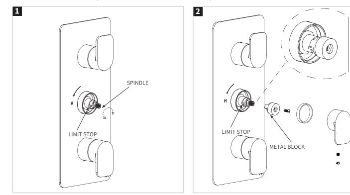
The temperature control handles on this product are factory set and should require no adjustment. However, if for any reason the handles and/or the cartridge is removed it is important the following procedure is followed.
