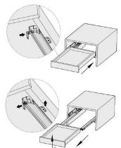
Pull out the drawer to its full extension, gently squeeze the locking levers outwards on both sides and pull the drawer off the runners at the front.
