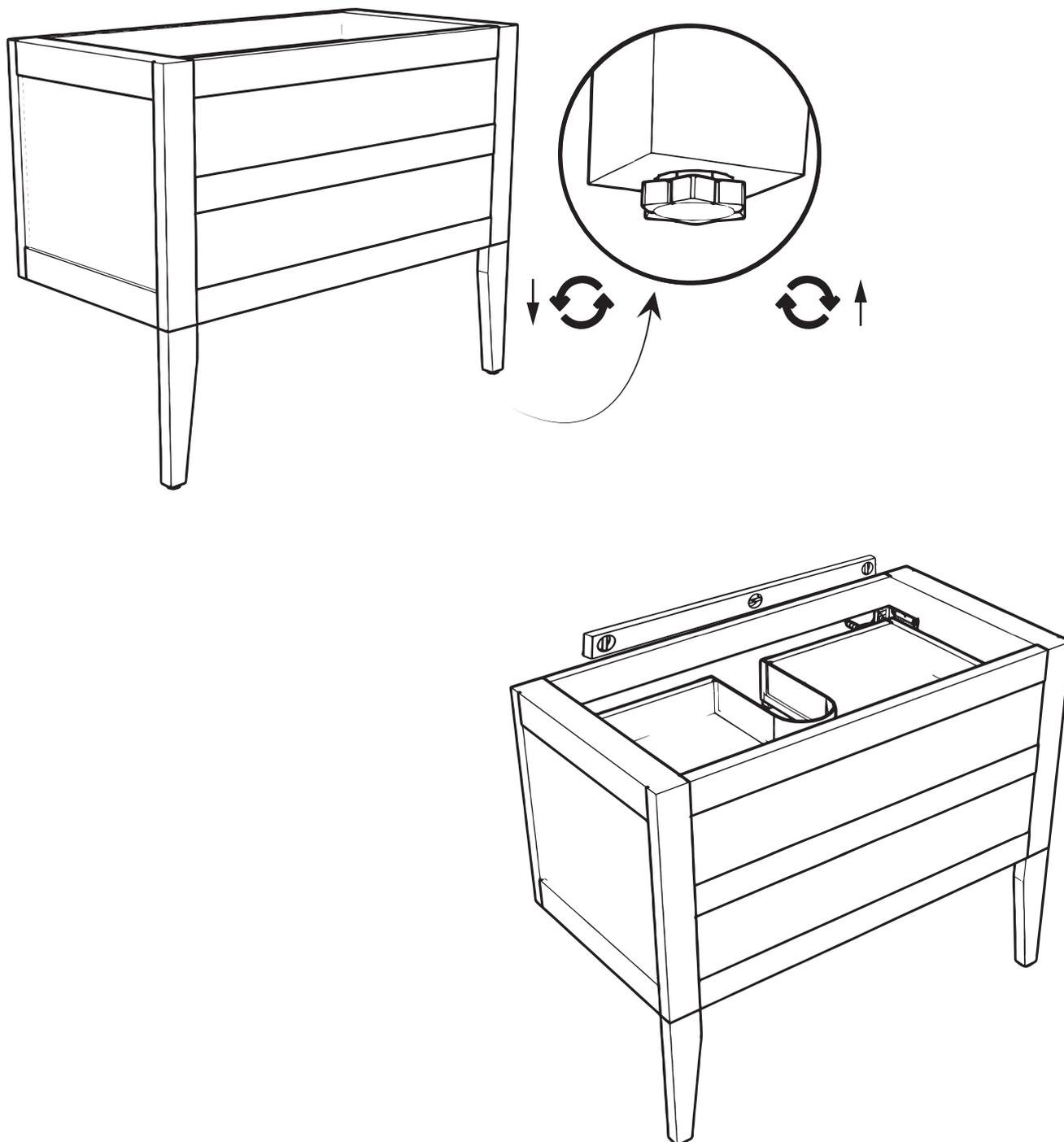
Remove the drawer border to insert the handle
