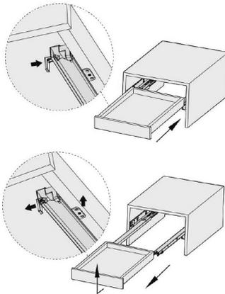
Pull out the drawer to its full extension, gently squeeze the locking levers outwards on both sides and pull the drawer off the runners at the front.
