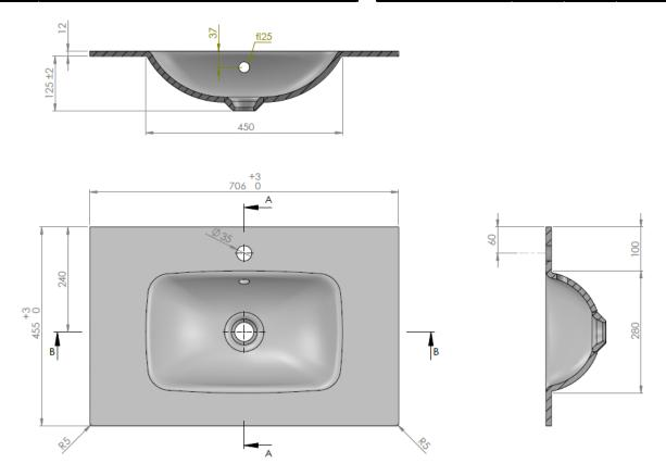
Sizes detailed could have a variation of about +/-5 % due to the changes to material characteristics during the firing processes. Exact measurements for individual installations can only be taken from the finished basin.
